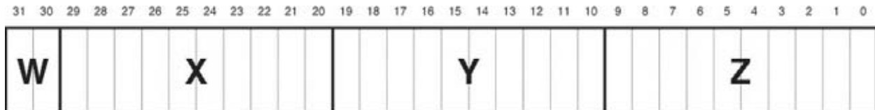
Figure 3.3 Packing of elements in a BGRA-packed vertex attribute
